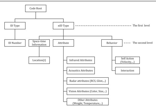
Fig. 1 The Tree-Code logical structure. Notice: this tree code structure is flexible which is convenient for adding high order levels, tree leaves, and extending new type in the 1st level or 2nd level. The ID type is compatible with all existing coding rules in the world, e.g. bar code, and EPC code
